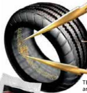
A tire with a heavy spot on the tread pulls the tire outwards, causing a force that results in vibration.
