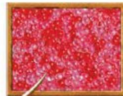
TECH PLUS microbeads are spread evenly around interior of the tire through centrifugal force.
